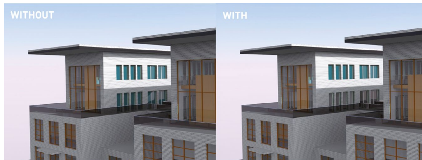
Figure 3 Somfy's Shadow management device manages the buildings response to shadows cast on it by neighbouring buildings, allowing only the windows/zones exposed to the sun to have their solar shading lowered.
