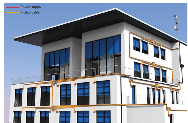
Figure 1 Integrating Somfy's animeo range into a buildings BMS/LMS takes the functionality of the building one step further, availing a range of comfort, energy savings and security functions.
